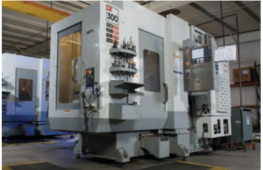
Our newest CNC machining centers produce a complete valve body and components to world class tolerances.
