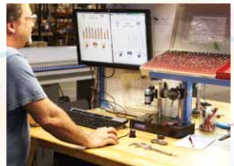
CNC machining centers are monitored continuously for accuracy and overall performance.
